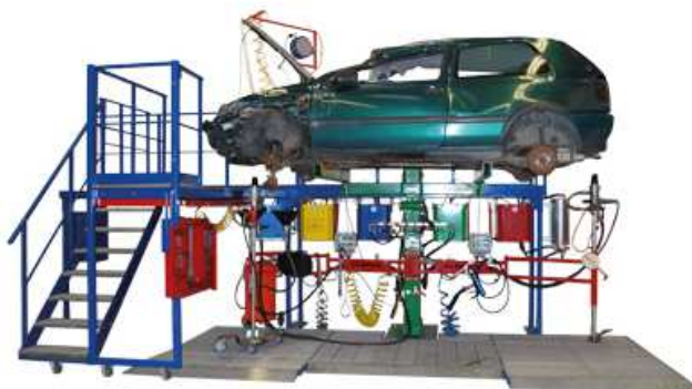
Figure 2: SEDA Single Station drainage system ( www.seda-international.com )
