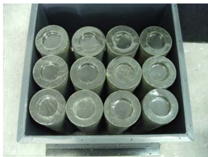
Figure 4. Adsorption filter in the form of a cluster group
