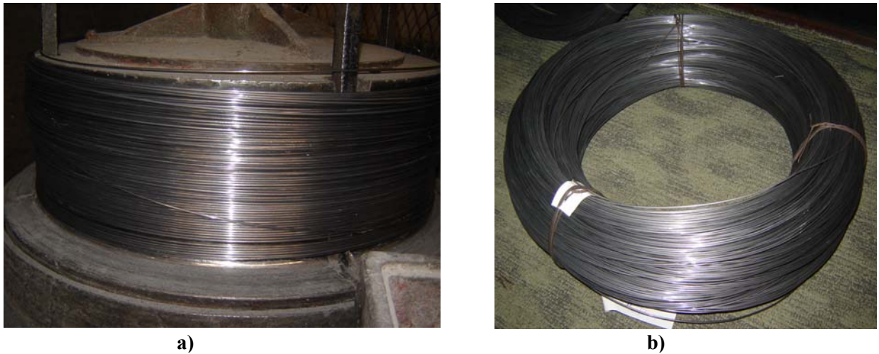
Figure 6. Appearance of flux-cored wire after drawing (ASCO VIDAK-Futog)
