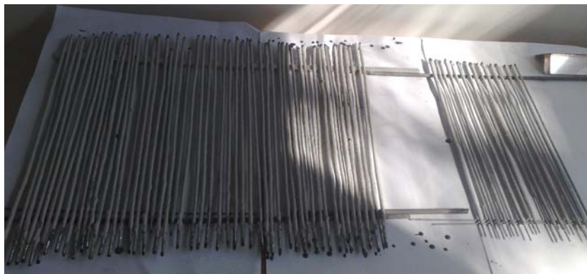
Figure 8. Appearance experimentally produced coated electrode with a core of solid and flux-cored steel wire
