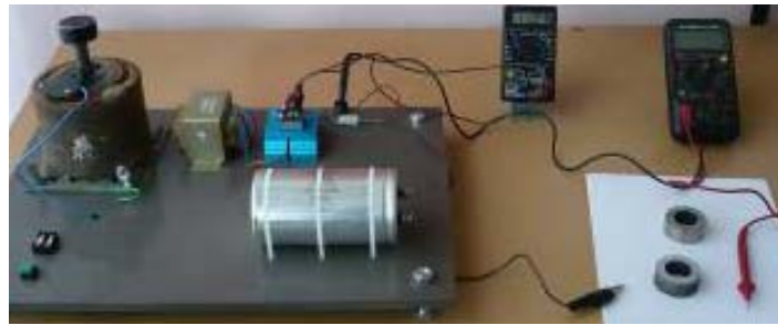
Figure 3. Rack developed for ohmic resistance measurement.
