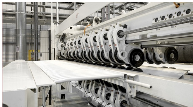
Figure 9. Modul longitudinal cutting machine for paper
