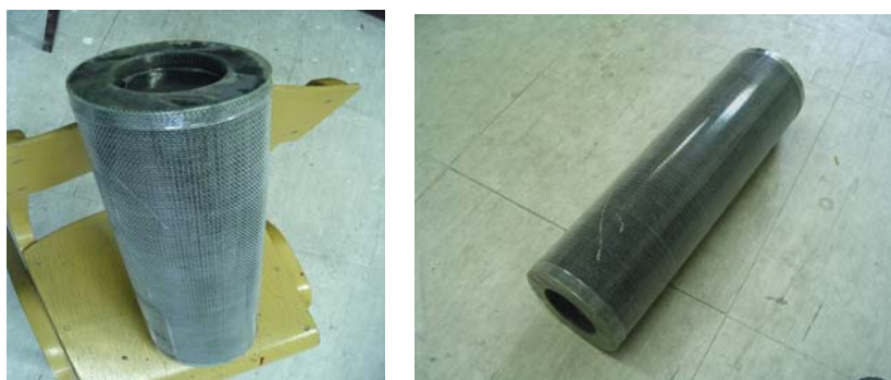
Figure 3. Cartridge with activated carbon.
