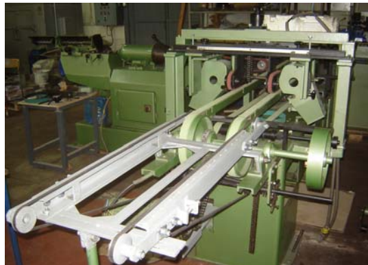
Figure 7. Layout of the experimental line for production of coated electrodes
