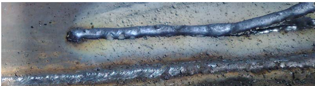
Figure 10. Appearance of trial surfacing with experimentally produced electrodes (a, b, c, d, e)
