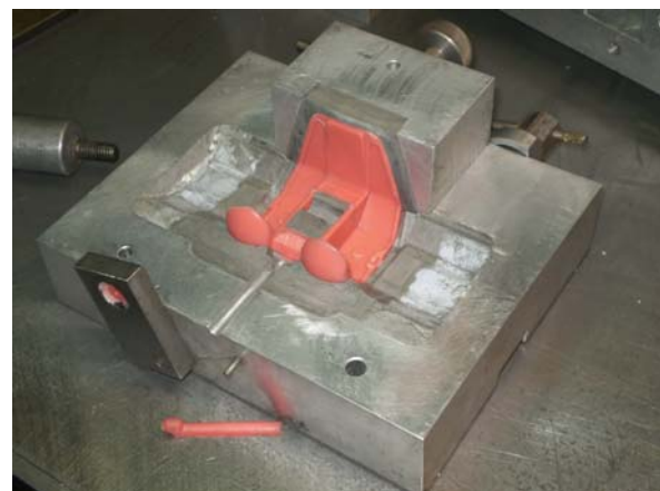
Figure 3. Disassembled tool with meltable wax model
