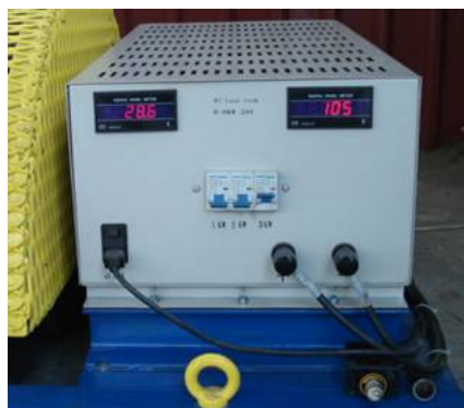
Figure 5. System for controlling DC loads 0-6 kW, 28 V
