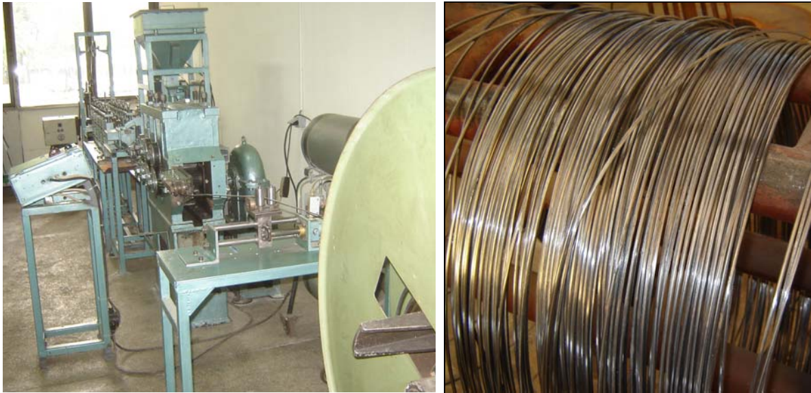
Figure 4. Layout of experimental line (a) for production of flux-cored wire (b)
