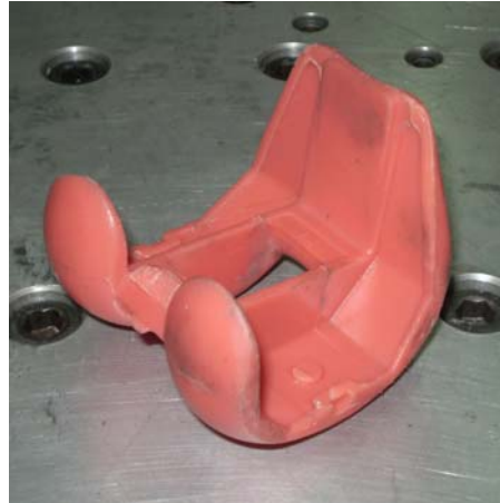
Figure 6. Meltable wax pattern of knee implant
