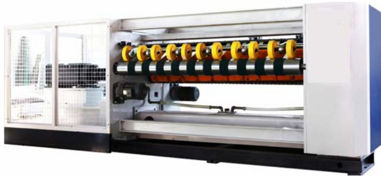
Figure 10. Transverse knife for cutting cardboard
