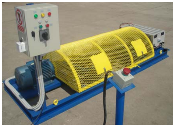
Figure 1. The laboratory stand with a closed protective fence
